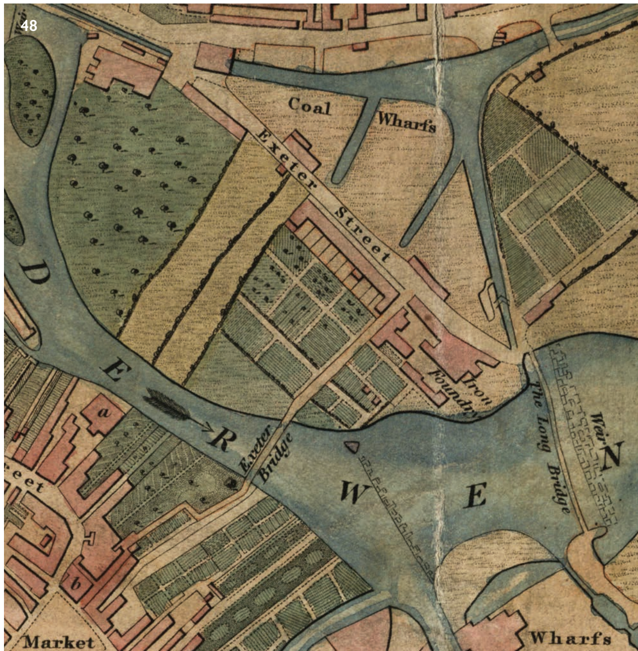
48: W. M. Rogerson's plan of 1819 (Derby maps no. 15 - reproduced with permission, Derby Local Studies and Family History Library). The east bank of the River is in a state of transition following the construction of the Derby Canal. Derwent Foundry lies between two weirs on the east bank, with rows of cottages along Exeter Street and cottagers garden allotments. Exeter Bridge is also evident and at this date was a timber structure.
