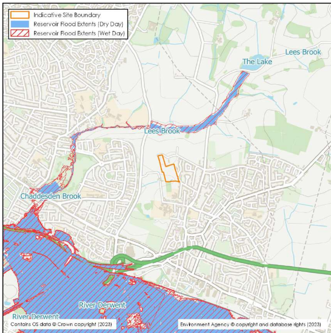
Figure 3.5: Reservoir Failure Flood Risk Map
