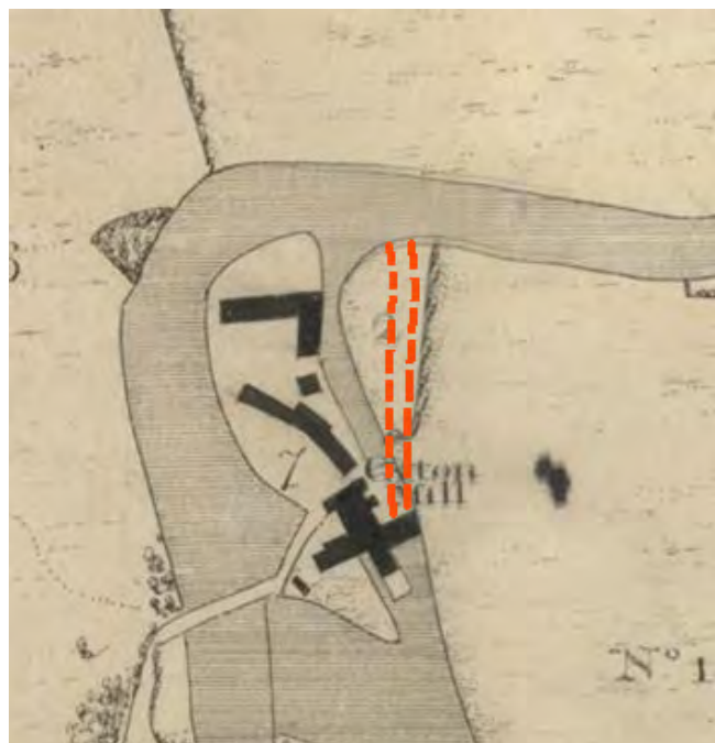
Figs.15 & 16 Comparison of the 1792 Outram plan and the Liberty plan of 1811. When orientated north (as above), the line of the leat on the Outram plan appears to be northerly and not located following the alignment of the curved building. Right - the dotted line overlaid on the Liberty map is suggested as a possible original alignment of the leat, as it corresponds with a north-south boundary marked on the 1811 plan and is the natural place for a long head race, as found at other early sites along the valley, such as Belper (Burton Weir) and Milford (Hopping Mill Weir and the original Foundry Weir).
