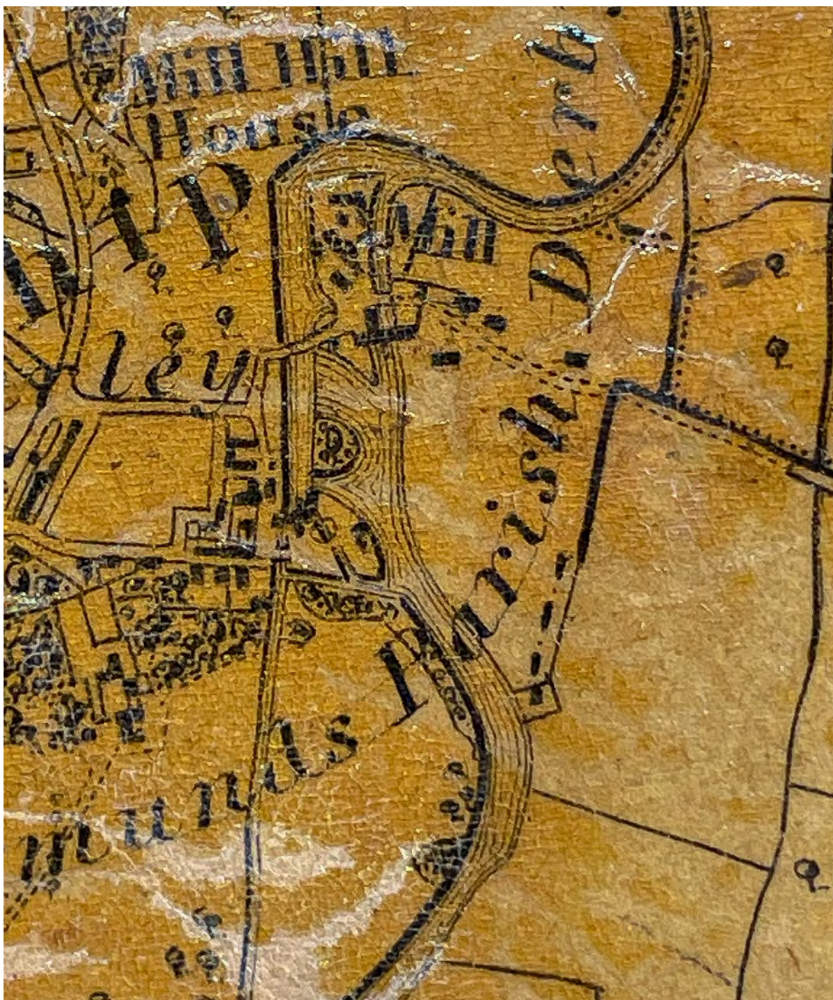
Fig.18 1835 Sanderson map – extract (DRO – D6572/1). The water is clearly marked and illustrated with contour lines flowing through sluices on the left bank above the bridge and the bank above the bridge is clearly built-out where it adjoins the sluices. The weir is not illustrated with its distinct curved shape for the northern straight-drop section.
