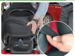
The seatbelt must be routed properly before tightening. Push down on the seat and pull the belt through to remove the slack and help tighten. Flick the belt at the beginning to check the tension; it should be tight.
