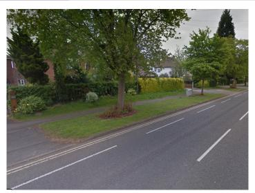
Currently the length of road from Palm Court Roundabout to Broadway has advisory cycle lanes. The proposal is to introduce mandatory cycle lanes and add light segregation to provide greater protection for cyclists. The cycle lanes will be 1.5m wide with an approx. 400mm buffer between cycle and other traffic.
